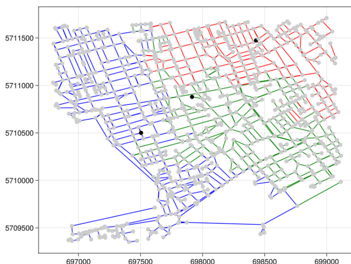
Fig. 4. Three districts of the network of London of 1000 of vertices on the data set of [3]. The depots are highlighted in the given figure.
