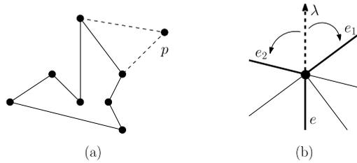
**Fig. 5.** (a) We can always connect a new vertex  $p$  outside the convex hull of  $S$  to two endpoints of some edge of the spanning cycle. (b) The set  $\{e, e_1, e_2\}$  is a valid triple of edges.
