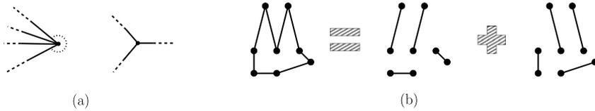
**Fig. 4.** (a) A vertex is valid if and only if it is not a reflex vertex of any face. (b) In a point set of an even size, every spanning cycle is the union of two edge-disjoint perfect matchings.
