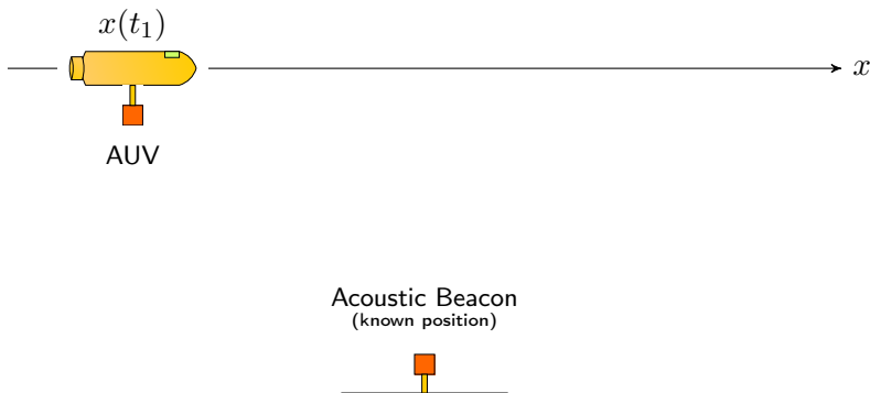
Figure : AUV's localization with an acoustic beacon on the seabed
